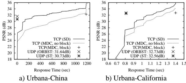
Figure 6: Delay-quality trade-offs between TCP delivery of transmitting SDC image data *pepper* to two remote sites at 12 noon their local time. (The behavior at other times is similar.)
