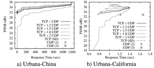
Figure 7: Delay-quality trade-offs of the combined TCP/UDP delivery of SDC/MDC data for *peppers* for the transmissions from Urbana to two remote sites at 12 noon their local time.
