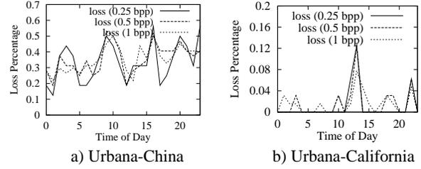
Figure 4: Loss rates of 16-, 32- and 64-packet transmissions from Urbana to two remote sites.
