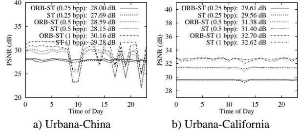
Figure 5: Comparisons of reconstruction quality in transmitting image *peppers* over a 24-hour period when each image was coded at, respectively, 0.25 bpp, 0.5 bpp, and 1 bpp, and placed in 16, 32, and 64 packets for transmission.
