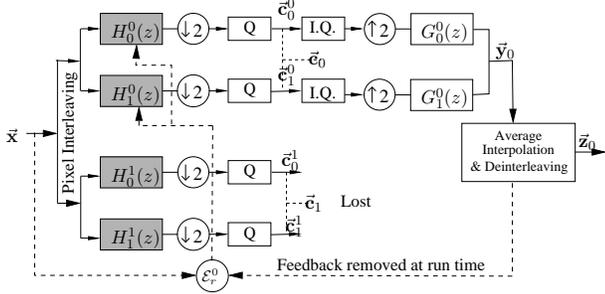
Figure 3: Basic building blocks of a modified codec. (The shaded block is our proposed ORB-ST.)
