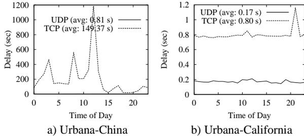
Figure 1: Round-trip delays of sending 64 UDP packets and the same data in TCP packets encapsulated in UDP ones to the UDP echo port of two remote computers. The experiments were carried out over a 24-hour period on April 8, 2001.
