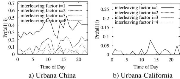
Figure 2:  $Pr(fail|i)$ , probability of bursty losses that cannot be recovered, conditioned on interleaving factor  $i$ , at different times on April 8, 2001.
