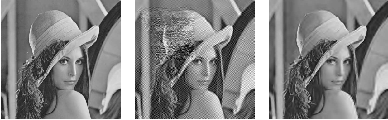
a) SDC by TCP (30.97 dB and 4.01 sec.) b) SDC by UDP (20.51 dB and 0.71 sec.) c) Proposed MDC by UDP (25.21 dB and 0.71 sec.)
