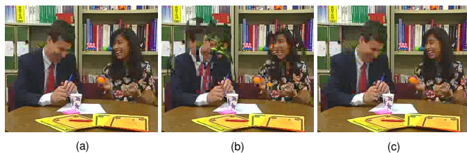
Fig. 8. Sample frame (the 55th frame) of Paris by the previous method under a) a loss-free environment (PSNR = 27.9 dB) and b) a lossy environment (PSNR = 22.0 dB), and c) by our proposed method under a lossy environment (PSNR = 27.3 dB).
