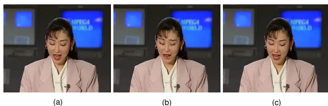
Fig. 7. Sample frame (the 88th frame) of Akiyo by the previous method under a) a loss-free environment (PSNR = 37.5 dB) and b) a lossy environment (PSNR = 31.9 dB), and c) by our proposed method under a lossy environment (PSNR = 37.9 dB).
