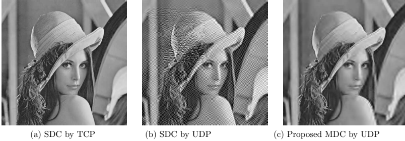
Figure 4.20 Quality-delay trade-offs in round-trip transmissions of lena compressed at 0.125 bpp by JPEG2000 between UIUC and Thailand. In UDP transmissions, two out of the eight packets were lost. Image (a) has a quality of 30.97 dB and a delay of 4.01 sec. Image (b) has a quality of 20.51 dB and a delay of 0.71 sec. Image (c) has a quality of 25.21 dB and a delay of 0.71 sec.
