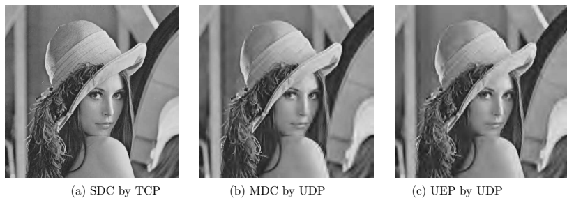
Figure 5.18 Quality-delay trade-offs in round-trip transmissions of lena compressed at 0.125 bpp by JPEG2000 between UIUC and Thailand. In UDP transmissions, two out of the eight packets were lost. Image (a) has a quality of 30.97 dB and a delay of 4.01 sec. Image (b) has a quality of 25.21 dB and a delay of 0.71 sec. Image (c) has a quality of 26.03 dB and a delay of 0.71 sec.
