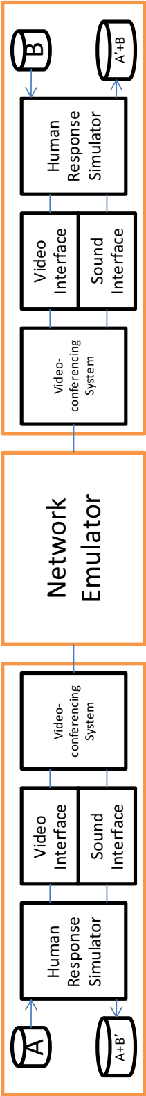
Figure 6.3: The architecture of RealTalk , an evaluation testbed for proprietary video conferencing systems.
